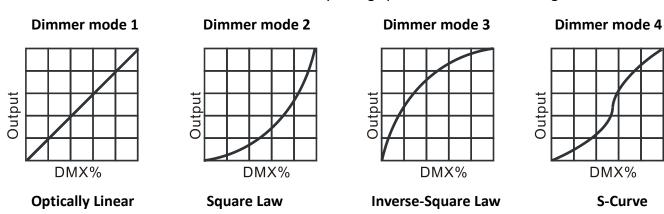
Mode 1(Optically Linear): The increase in light intensity appears to be linear as DMX value is increased. Mode 2(Square Law): Light intensity control is finer at low levels and coarser at high levels.
