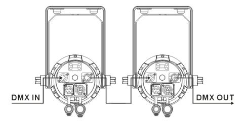
Connect the fixture together in a "daisy chain" by XLR plug cable from the output of the fixture to
